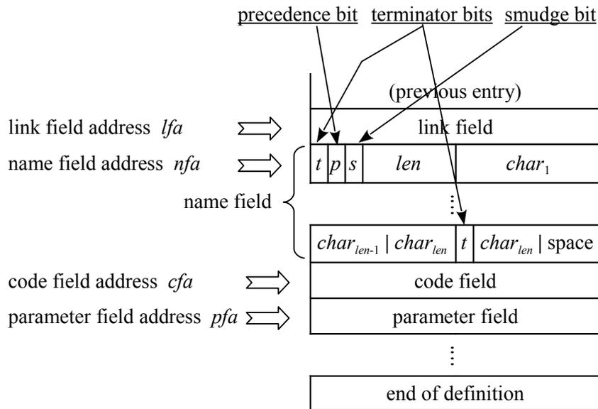
At the least, each entry contains a link field (1 cell), a name field (1 – 16 cells), a code field (1 cell) and a parameter field ( $n \geq 1$  cells).
